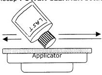
4. Clean record by moving applicator in a sweeping motion. Follow the record grooves around the record two times. Collect dust particles onto the applicator.
