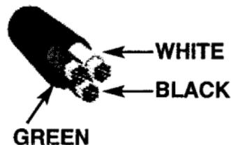
Make certain there is no wire insulation clamped inside any terminal, and there are no stray wire strands outside the terminals. Tighten the terminal screws to 12 in-lbs torque. Do not over tighten.
