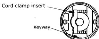
3. Cable Preparation: Select the proper end of the cord for the plug or connector. Feed the cable through the housing and strip the cord as shown below. Make sure the wire is clean, and a bright copper color. If necessary, cut back the wire until clean wire is uncovered. Do not solder the ends of the wire.
